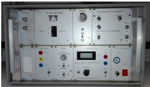
First German MCC-IMS for breath analysis from ISAS (2001/2002)
